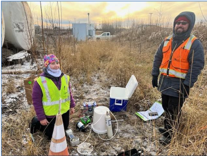
Air Force contractors conducting soil gas sampling for petroleum contaminants at Site ST005 Area C.
